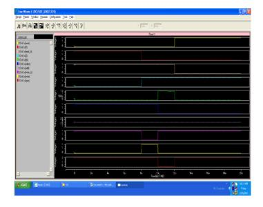
Figure 9 : READ Operation - 12T SRAM
