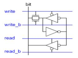
Figure 3: Structure of 12 T SRAM
