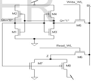
Figure 2 : Structure of 8T SRAM
